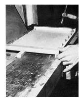
Fix the top (14ii) and the bottom (14iii) edges with 3/4" brass pins to what will be the outside of the centrecase (the bottom pieces are the two beveled strips. The bevel goes at the bottom where the packing pieces protrude slightly). The top and bottom edges are pinned and glued flush with the outside edge of the centrecase.
