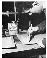
Coat all surfaces that will be inside the centreboard case and exposed to water with 2 or 3 coats of epoxy. Sand between coats and make sure that there is a smooth finish.
