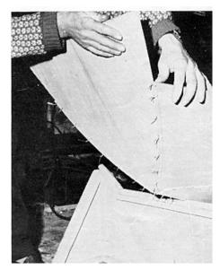
Fix one side of the fore transom to the corresponding bottom panel using the copper wire pieces to the same tension as that on the aft transom. Note that the ends of the bottom are curved, but when they are bent around the transom the two curves cancel each other out and appear to straighten.
