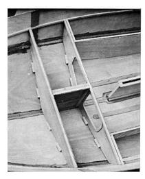
The side tank sides (13) fit against the upright pieces on the aft and storage bulkheads. These panels may need to be trimmed slightly to fit. Bevel the bottom outside edges. They must fit snug. (In some cases the top batten (13i) is not fixed to the side tank panels. Fix with glue and copper nails.) Drill a 15 mm +/- 5 mm drain hole in what will be the lowest position (check appropriate size vs. the supplied fittings)
