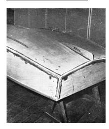
Cut two lengths of tape 1" longer than the skeg. Apply an extra coat of resin to the area which the skeg will cover, screw the piece into position set the nail and apply the tape and resin to bond it down to the boat on either side.
