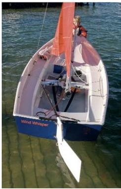
**Above and left** The cockpit of the new Mk3 Mirror (above) – compared to the earlier model (left) – incorporating a curved foredeck and raised mast foot on the Mk3, plus calf-friendly angled sidetank edges.
